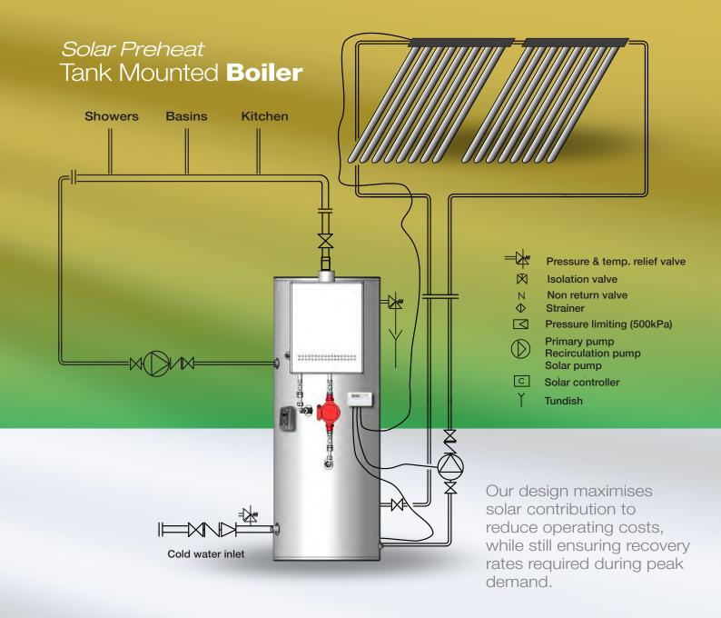
The Wilson Solar Preheat range is designed from the ground up for specific functions that include stand alone storage tanks, combination units for Solar/Gas or Electric boosted systems.
